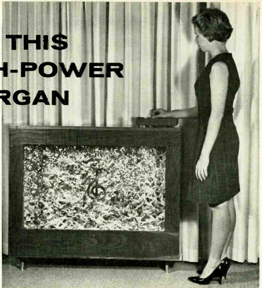
Author's Colorgan is housed in walnut cabinet. Light display is reflected from crumpled aluminum foil.
