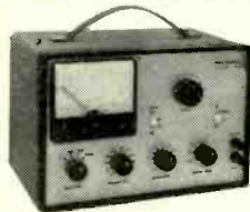
New Model 378 Audio Generator. Near-distortionless sine wave generator (< 0.1% 20-20,000c) providing fast, convenient, switch-selection of frequencies from 1c to 1,000c (1c steps 10c-100c, 10c steps 100c-1kc, 100c steps 1kc-10kc, 1kc steps 10kc-100kc). 8-pos. 10db/step output attenuator & fine attenuator. Output meter (4 1/2" 200ua) with 8 voltage ranges & db scale. $44.95 kit, $64.95 wired.
