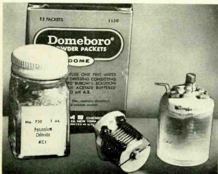
The ingredients and the finished product: potassium chloride (used to make the hydroxide), aluminum acetate, a small all-aluminum variable capacitor; and a finished, formed variable electrolytic.
